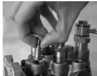
Remove the delivery valve and gasket.
