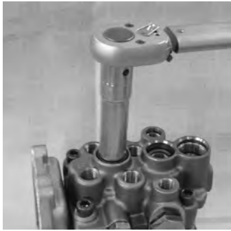
Fasten the plug, (distribution shaft).
