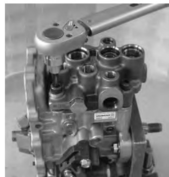
Install the hydraulic head CMP fastening bolt.
