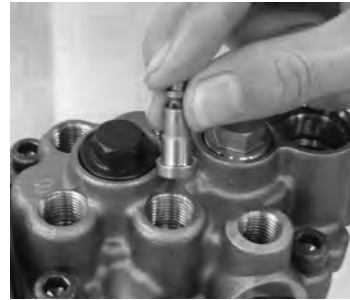
Install the delivery valve CMP.
