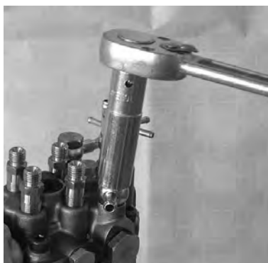
Remove the joint, (FO inlet pipe).
