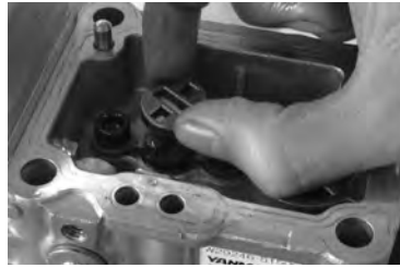
Remove the joint, (distribution shaft).
