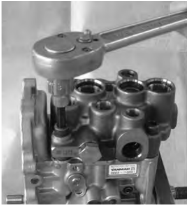
Remove the hydraulic head CMP fixing bolt.
