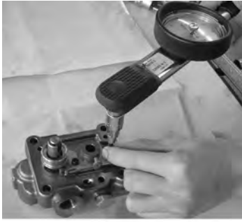
Install the rack guide fastening bolt.
