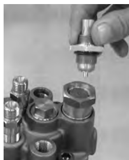
Install the thermo-element with new O-ring.
