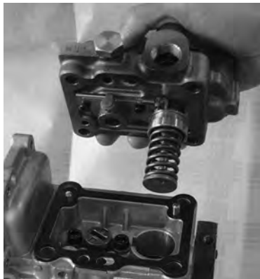
Remove the hydraulic head CMP.
