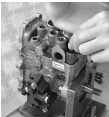
Install the hydraulic head CMP.
