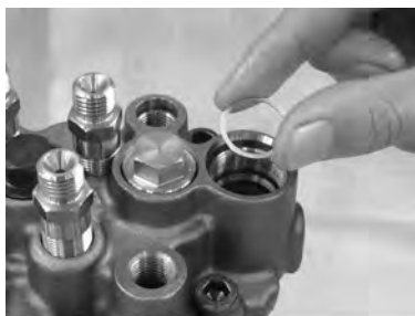
Install the new packing, (timer).
