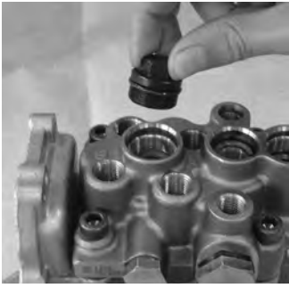
Install the plug, (distribution shaft).
