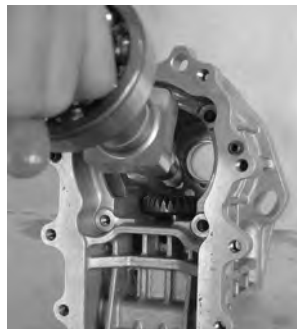
Install the camshaft.
