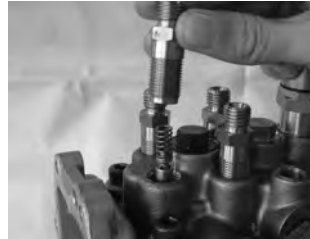
Remove the delivery valve and gasket.
