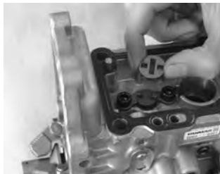
Install the joint, (transmission snart).
