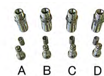
Delivery valve parts disassembled. (Take care not to mix these with other parts on reassembly. Reassemble these to the original port as a set.)
