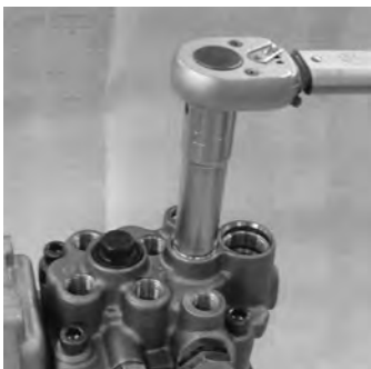
Fasten the plug, (barrel).
