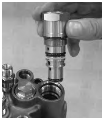
Install the holder with new O-ring, (timer).
