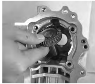
Install the transmission shaft CMP.
